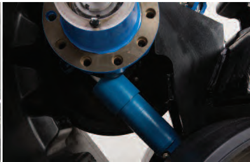
Integrated accumulator/tensioner for belt tension adjustment.
